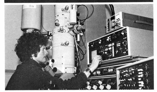
FOR BETTER SCRUTINY of the material under study, Rob Allen (8316) adjusts the signal mixing system on the STEM to electronically mix different images of the sample.
